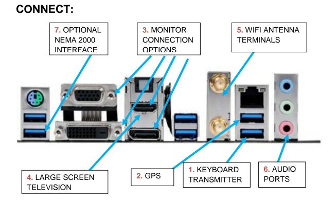
**1.** Connect a wireless keyboard transmitter to the indicated USB port.
